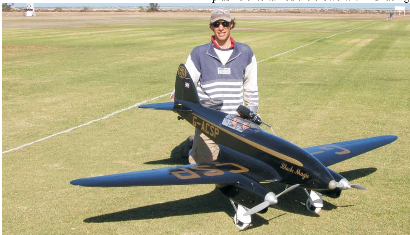
Gorgeous De Havilland DH 88 Comet built from scratch and raced by South Australian Richard Mudge. A pair of OS 160FX engines home built retracts and a finish you could shave from
